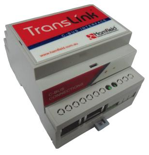
The Translink group of products provide a gateway into a Clipsal C-Bus network, and present the user with an easy to use interface with real time viewing and control of their network
