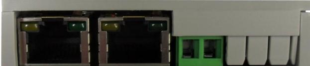
Figure 2 C-Bus Connections
